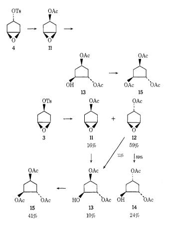
of cis tosylate 3, both cis and trans acetates 11 and 12 are initially produced in the amounts of 16 and 59%, respectively. Both acetates decompose completely during the course of the reaction, 11 giving only 13 and 12 giving 13 and 14 in a 1:8 ratio. This results in a
